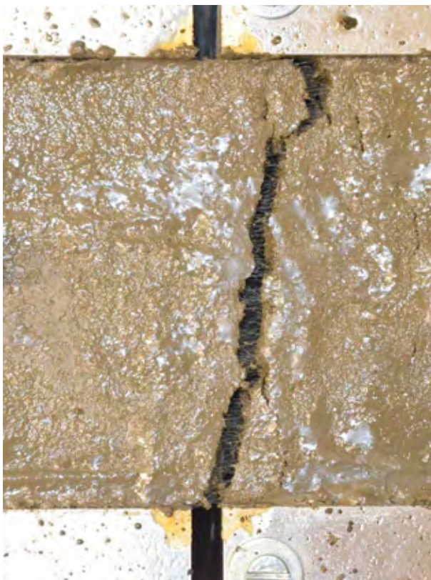
Figure 2: Direct tensile test on fresh concrete clearly showing the fibres bridging the crack even after extensive crack opening.
