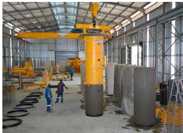
Vertically cast pipe production.
