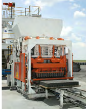
Birkenmayer recently exported their largest brick/block making machine, the HB68, into Africa for Zimbabwean client, Vaka Afrika.
