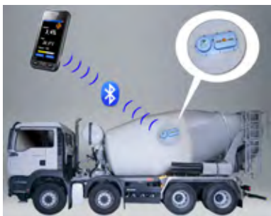
Readymix truck with a receiver module (above) and below, ready-mix truck with an external receiver.
