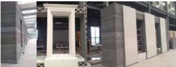
3D printed components for WinSun's structures are built off-site.
