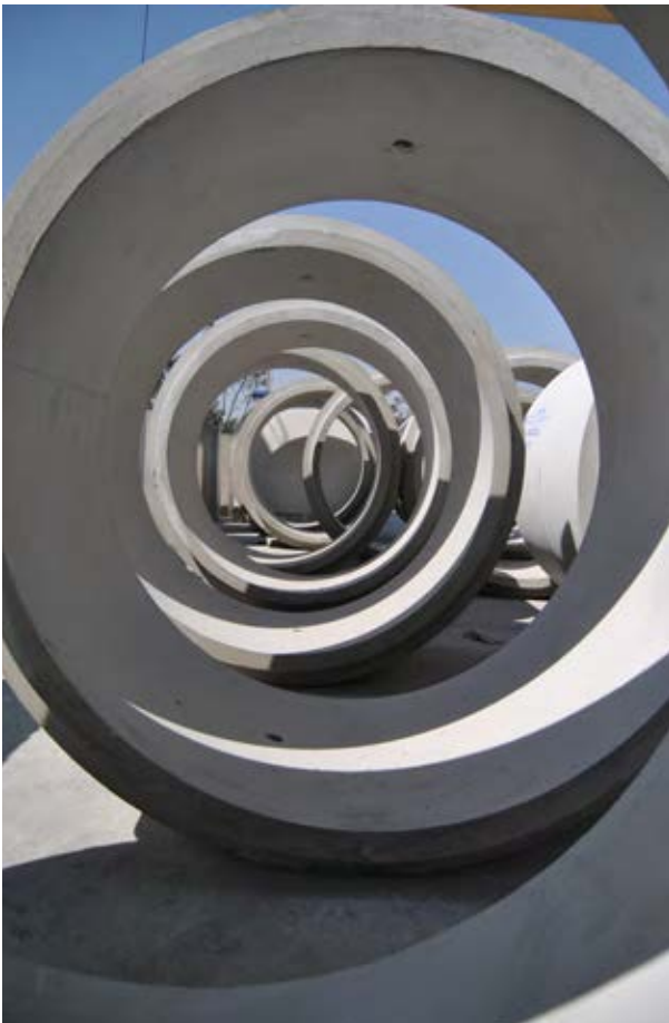
The Rocla jacking pipes on site at their Roodepoort factory.
