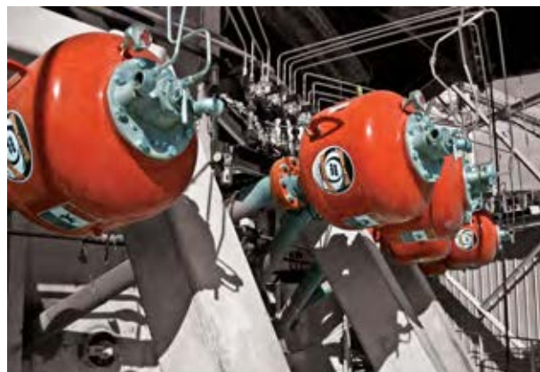
New air cannon valves from Martin Engineering produce about twice the blast force of the previous valve generation, from approximately half the compressed air volume.
