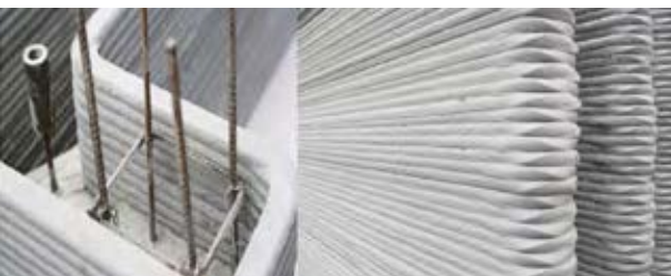
3D printed components for WinSun's structures are built off-site.
