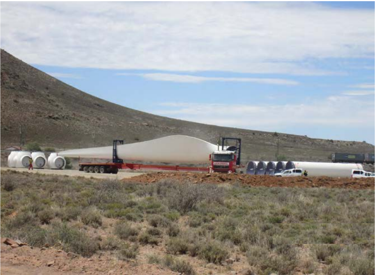
The vehicles on the right show the massive size of the turbine blades which had to be transported by road on vehicles up to 55 m long.
