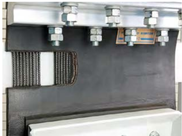
The new belts for the heavy-duty high capacity belt bucket elevators can be designed with a tensile load up to 3,300 N/mm.
