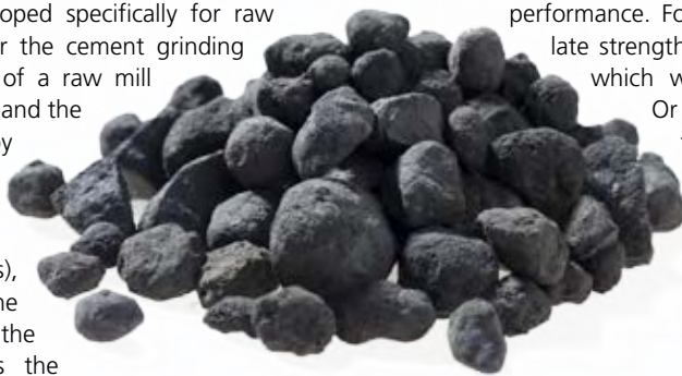
Clinker production is the most energy-intensive part of the cement-making process. Chryso activators help reduce clinker content, which cuts carbon emissions and carbon-tax costs.
