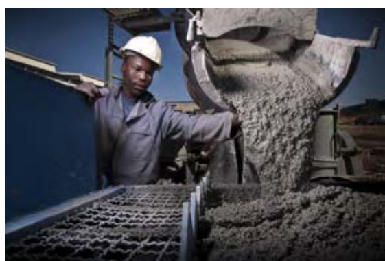
Another concrete trend is thermal concrete, which comprises cement infused with expanded polystyrene (EPS) balls. Thermal concrete is lightweight, with a high insulating factor and is ideal for roofs.
