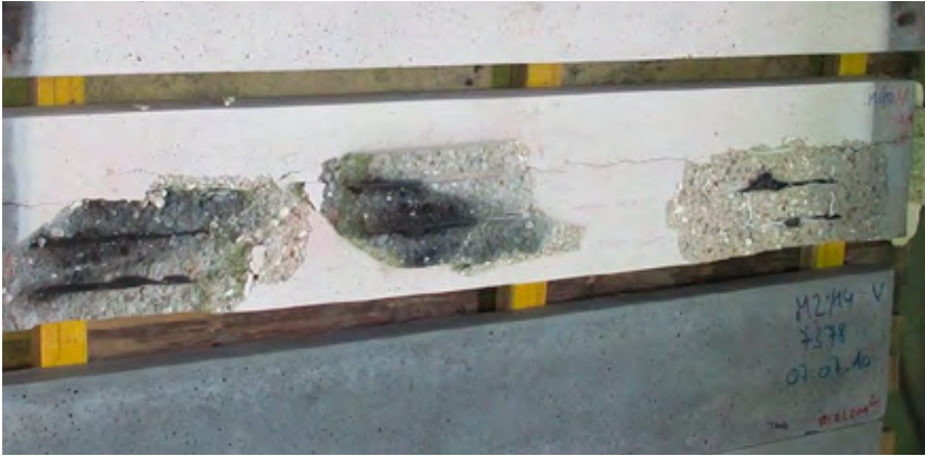
Researchers at EMPA tested walls with and without SAP using a radiant heater. Those without SAP exhibited much more severe cracking and flaking.
