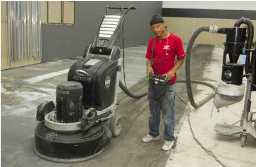
The remote controlled HTC 800 RX grinder with its operator. Polishing process stage 1 started.
