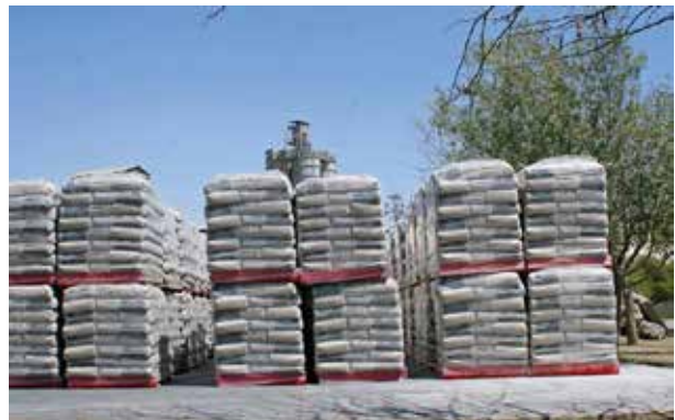
AD*STAR sacks palletised and stacked for storage outdoors. (picture courtesy of PPC Cement)
