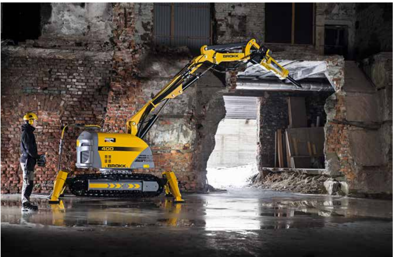
The Brokk 400 remote-controlled demolition machine features a robust, three-part boom that can operate at angles of up to 30° and reach 6,7 m horizontally and 7.3 m vertically.
