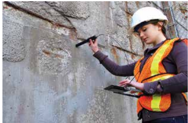
The Humboldt Giatec Cell is a tablet/smartphone-based NDT probe.
