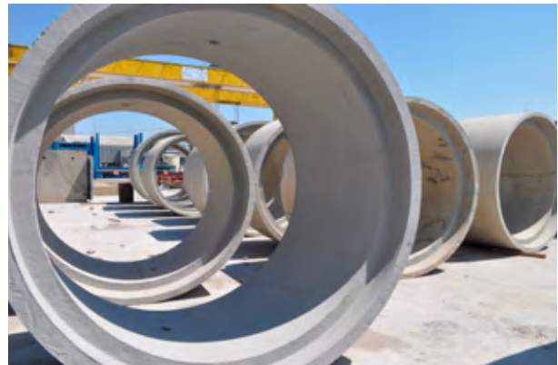
Jacking pipes with a 2,250 mm diameter at Rocla's precast manufacturing facility in Roodepoort.
