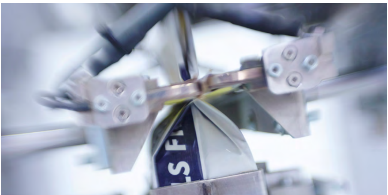
The ROTO-PACKER® ADAMS MINI small-bag packing machine, based on the proven ADAMS® technology, fills powder products into compact PE bags, reaching speeds of up to 600 bags/hr at steplessly selectable weights from 1 to 10 kg.
