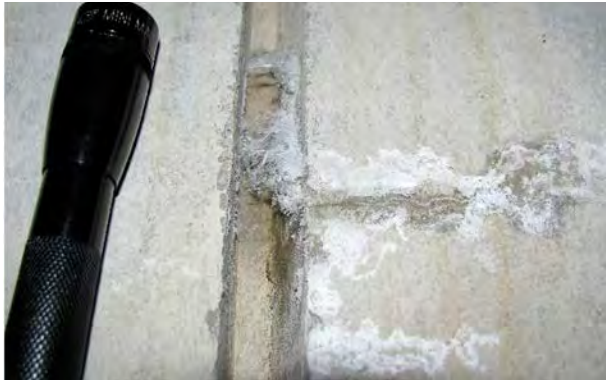
Kryton Crystal Growth can self-heal cracks guaranteed to 0.5 mm and in some cases 0.7 mm.
