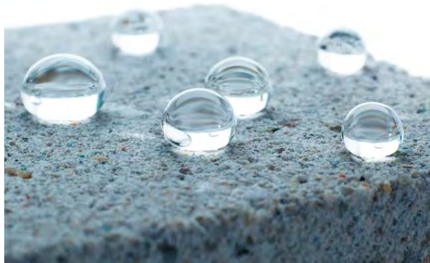
The beading performance of polysiloxanes.
