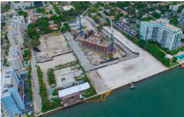
Water everywhere: These views of the Paraiso Bay construction site show its proximity to the Atlantic Ocean, which explains the high water table.
