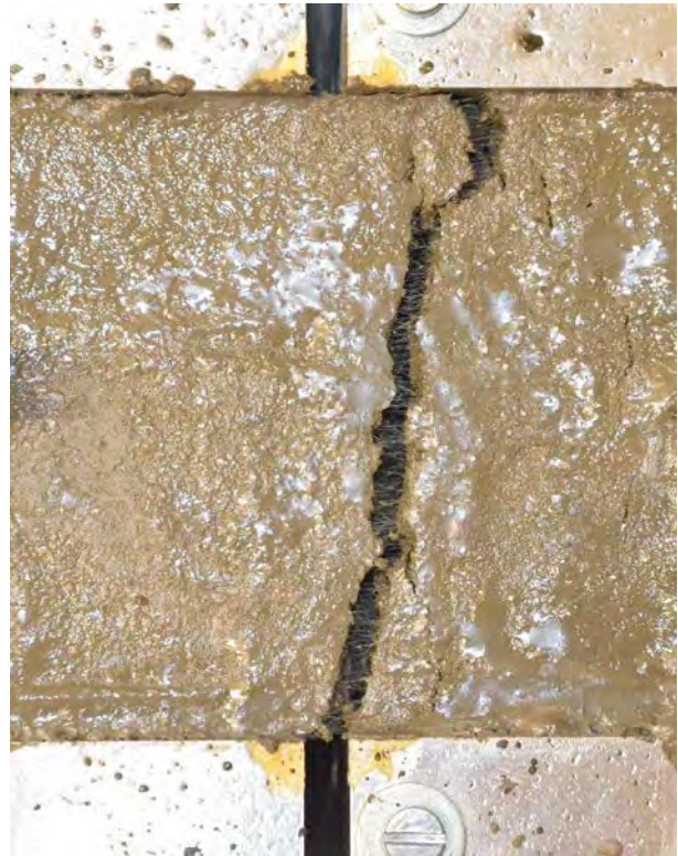
Direct tensile test on fresh concrete clearly showing the fibres bridging the crack even after extensive crack opening.
