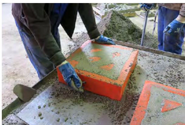
Filling the mould on a vibrating table.
