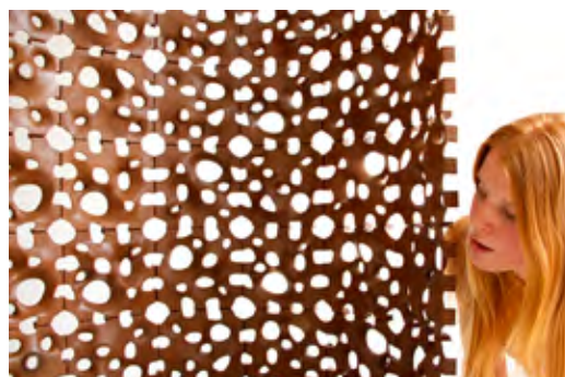
Page 48 - This Walnut Screen was 3D printed using hardwood sawdust fused with a special glue to create a stunning room divider.
