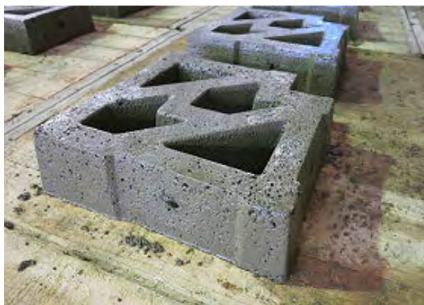
Freshly demoulded block with 10-mm holes.
