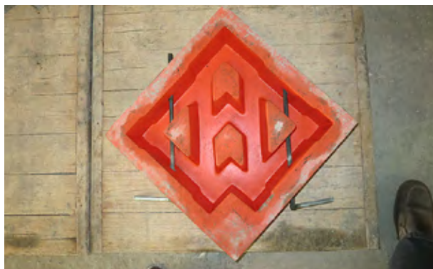
Mould box with rods.
