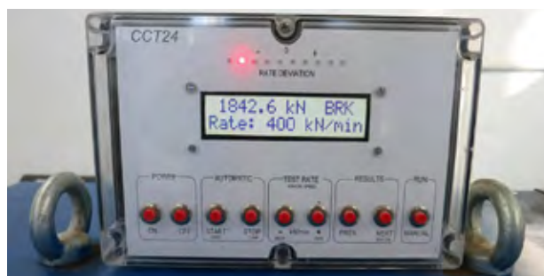
Compressive strength testing.
