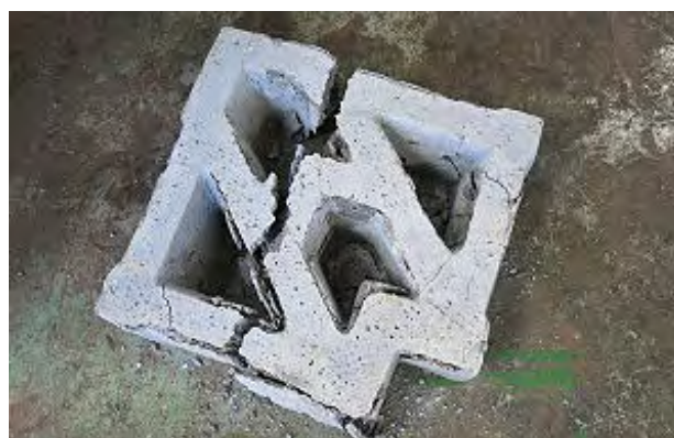
Crushed block after testing.
