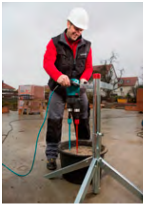
The handheld power mixers enable users to create homogenous mixes.
