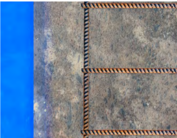
Crystalline technology turns porous concrete into an impermeable barrier, resulting in a structure with reduced cracking, self-sealing and waterproofing abilities that provide a powerful defense against water damage and corrosion of reinforcing steel.
