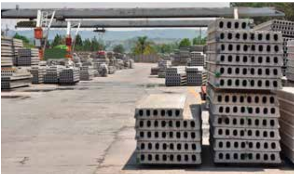
Reinforced hollow-core slabs prior to delivery at Echo Floors' storage yard.
