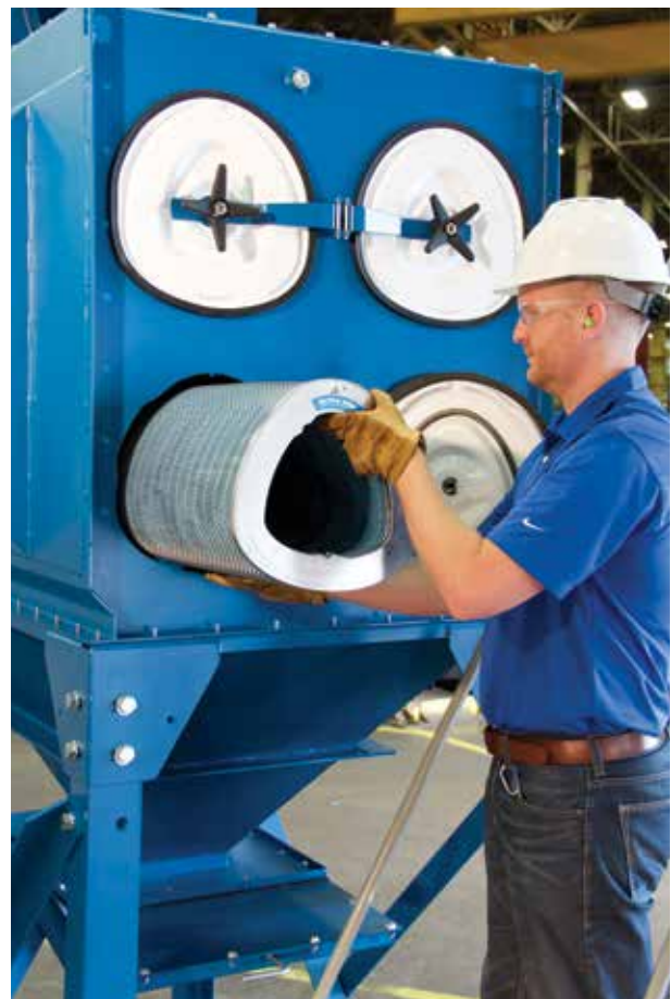
Downflo® Evolution (DFE) filter change out in a downflow collector
