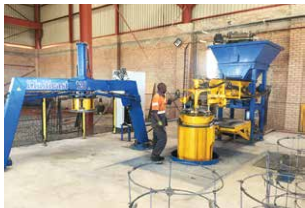
VIHY Multicast SCV 120 is a versatile vibration machine for production of manholes and short pipes up to 1200 mm diameter.
