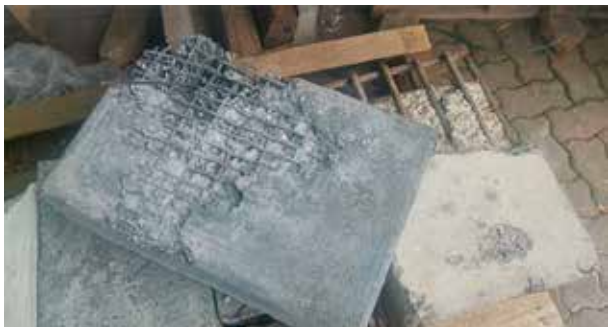
100-MPa geopolymer concrete with metal shavings after 200 hits.
